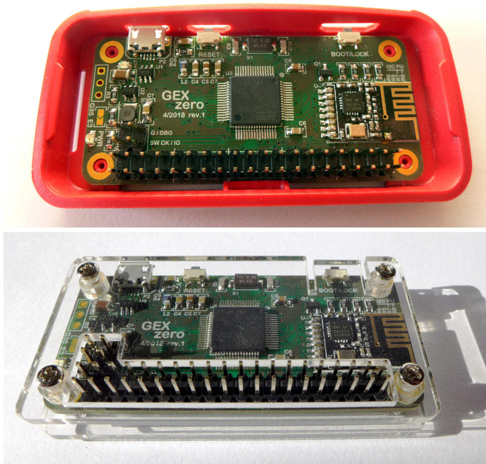
Figure 15.3: GEX Zero in the official Raspberry Pi Zero case, and an aftermarket acrylic case. The acrylic case is a better choice, as the button and the side connector are easier accessible, and the pin-out diagram on the back side of the board can be read without removing it.
