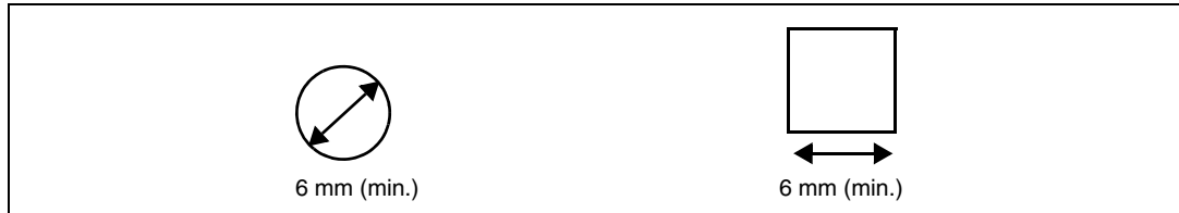
Figure 13. Recommended electrode size
