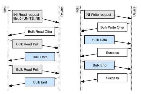
Figure 10.1: A diagram of the bulk read and write transaction.
