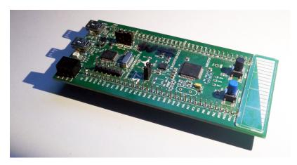
Figure 2.1: A Discovery development board with the STM32F072 microcontroller
