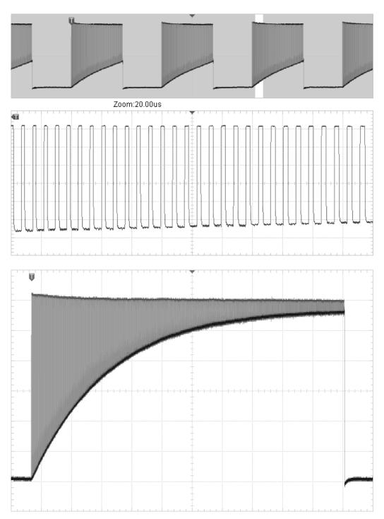
**Figure 8.8:** A voltage waveform measured on the touch sensing pad. The bottom side of the envelope equals the sampling capacitor's voltage—this is the phase where both capacitors are connected. The detailed view (middle) shows the individual charging cycles. The bottom screenshot captures the entire waveform after the analog comparator was disabled.
