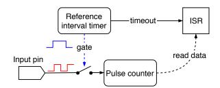
**Figure 8.1:** Direct frequency measurement method
