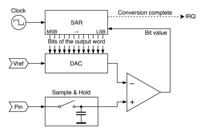
Figure 8.4: A diagram of the SAR type ADC
