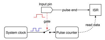
Figure 8.2: Reciprocal frequency measurement method
