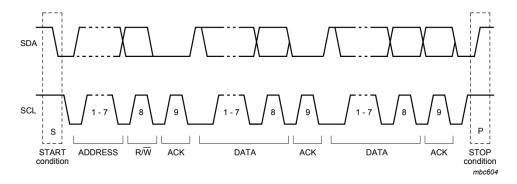
**Figure 7.3:** An I2C message diagram. The frame starts with a start condition and stops with a stop condition, defined by an SDA edge while SCL is high. The address and data bytes are acknowledged by the slave by sending a 0 on the open-drain SDA line in the following clock cycle. A slave can terminate the transaction by sending 1 in place of the acknowledge bit. (Diagram taken from the I2C specification UM10204 by NXP Semiconductors)
