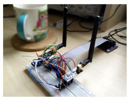
Figure 11.1: Test setup with a GEX prototype controlling two nRF24L01+ modules
