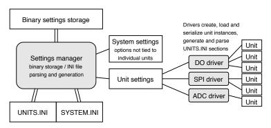
**Figure 9.2:** Structure of the settings subsystem
