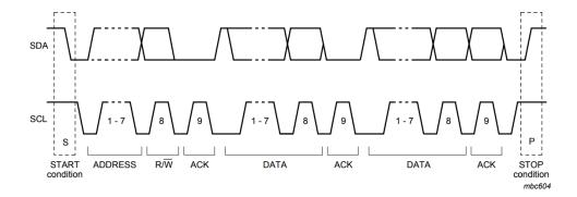
**Figure 7.3:** An I<sup>2</sup>Cmessage diagram. The frame starts with a start condition and stops with a stop condition, defined by an SDA edge while the SCL is high. The address and data bytes are acknowledged by the slave by sending a 0 on the open-drain SDA line in the following clock cycle. A slave can terminate the transaction by sending 1 in place of the acknowledge bit. (*Diagram taken from the I*<sup>2</sup>C specification UM10204 by NXP Semiconductors)
