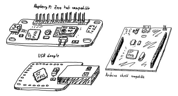
**Figure 2.2:** A sketch of three possible form factors for the GEX hardware prototype. Note the ESP8266 module which was considered as an option for wireless access but was eventually not used due to it's high current usage, unsuitable for battery operation.
