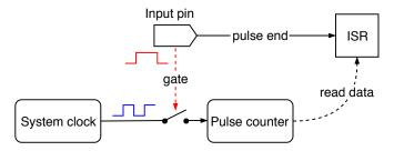
Figure 8.2: Reciprocal frequency measurement method
