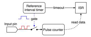
Figure 8.1: Direct frequency measurement method
