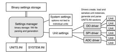
Figure 9.3: Structure of the settings subsystem
