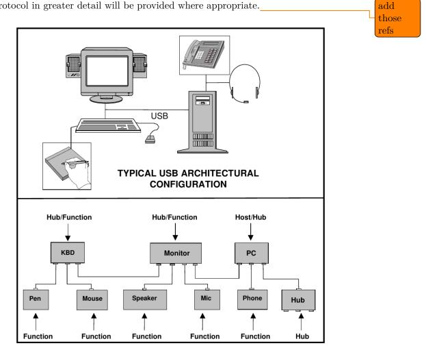
**Figure 4.1:** A diagram from the USB specification rev. 1.1 showing the hierarchical structure of the USB bus; the PC (Host) controls the bus and initiates all transactions.
