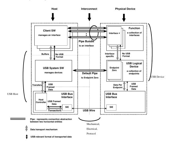
Figure 4.2: A detailed view of the host-device connection (USB specification rev. 1.1)
