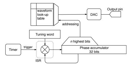
Figure 8.6: A block diagram of a DDS-based waveform generator
