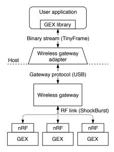
**Figure 14.2:** Wireless connection block diagram
