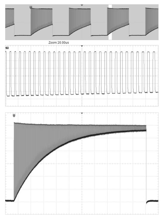
**Figure 8.9:** A voltage waveform measured on the touch sensing pad. The bottom side of the envelope equals the sampling capacitor's voltage—this is the phase where both capacitors are connected. The detailed view (middle) shows the individual charging cycles. The bottom screenshot captures the entire waveform, left to continue until a timeout, after the analog comparator was disabled.
