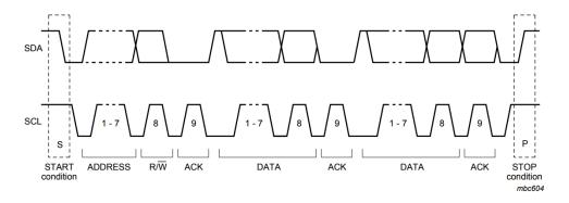
Figure 7.4: An I<sup>2</sup>C message diagram (taken from the  $I^2C$  specification [33])
