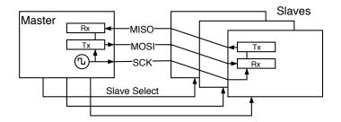
Figure 7.3: A SPI bus with 1 master and 3 slaves, each enabled by its own Slave Select signal
