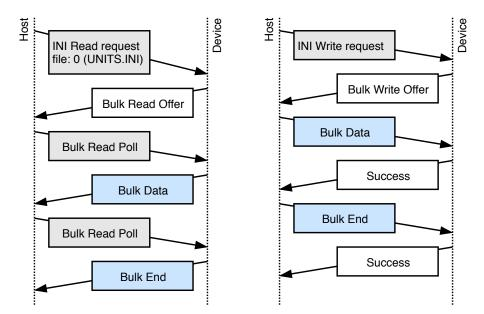
Figure 12.2: The bulk read and write transactions
