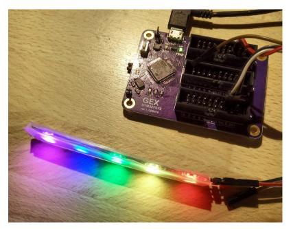
Figure 7.6: GEX prototype driving a strip of 5 NeoPixels
