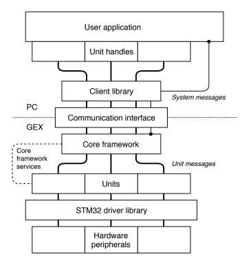
Figure 9.1: The "GEX stack", from a user application down to hardware
