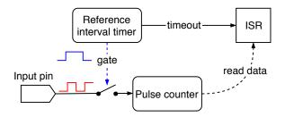
Figure 8.1: Direct frequency measurement method
