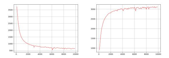
**Figure 17.2:** Frequency response of two complementary passive RC filters, captured by GEX controlled with a Python script. X: frequency (Hz), Y: peak-to-peak voltage as a raw ADC word
