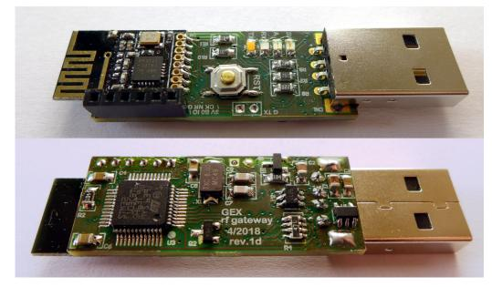
Figure 15.5: The wireless gateway (top and bottom side)
