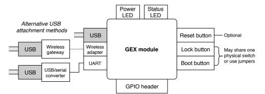
Figure 9.2: Physical user interface of a GEX module
