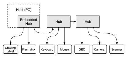
Figure 4.1: The hierarchical structure of the USB bus
