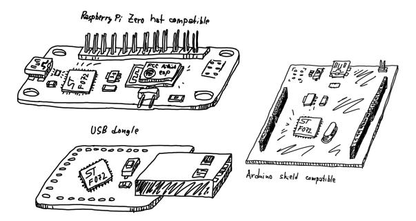
Figure 2.2: A sketch of three possible form factors for a GEX hardware realization
