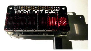
**Figure 16.1:** GEX Zero with the Micro Dot pHAT add-on board, showing a test pattern defined in a Python script
