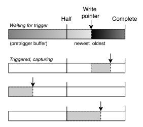
**Figure 13.4:** Principle of DMA-based ADC sampling. The buffer is continually filled with new samples; when the triggering condition is hit, the historical records from the buffer are sent as a pre-trigger buffer, and a block capture begins. The following samples are sent to the host when either half of the buffer is filled, or the required number of samples have been sent. The sampling never stops, ensuring a pre-trigger buffer is always ready.
