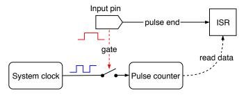
Figure 8.2: Reciprocal frequency measurement method
