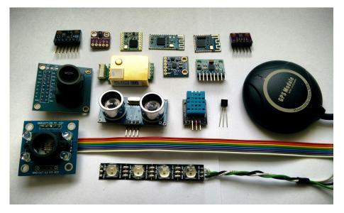
**Figure 1.1:** A collection of intelligent sensors and devices, most on breadboard adapters: (from the top left) a waveform generator, a gesture detector, a LoRa and two Bluetooth modules, an air quality and pressure sensor, a  $CO_2$  sensor, a digital compass, an accelerometer, a GPS module, a camera, an ultrasonic range finder, a humidity sensor, a 1-Wire thermometer, a color detector, and an RGB LED strip
