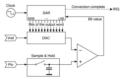
Figure 8.4: A diagram of the SAR type ADC
