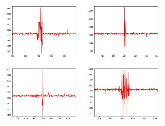
**Figure 17.6:** Lightning strike-generated bursts of energy captured by the ADC unit. Note the X-axis value 500 where the bursts start: that was the configured pre-trigger length
