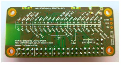
Figure 15.4: Pin assignment diagram on the back side of GEX Zero
