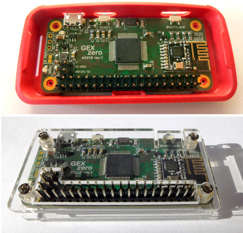
Figure 14.2: GEX Zero in the official Raspberry Pi Zero case and an aftermarket acrylic case
