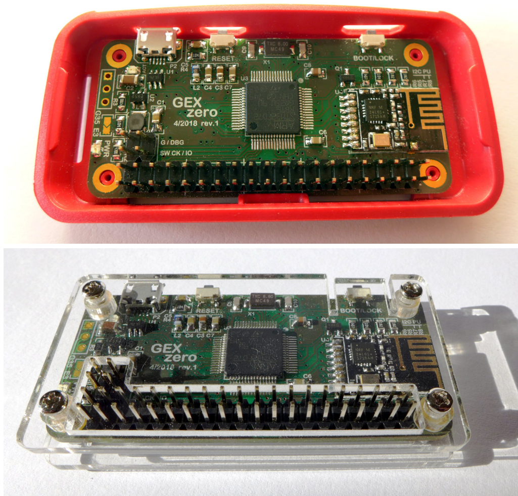
Figure 12.3: GEX Zero in the official Raspberry Pi Zero case and an aftermarket acrylic case
