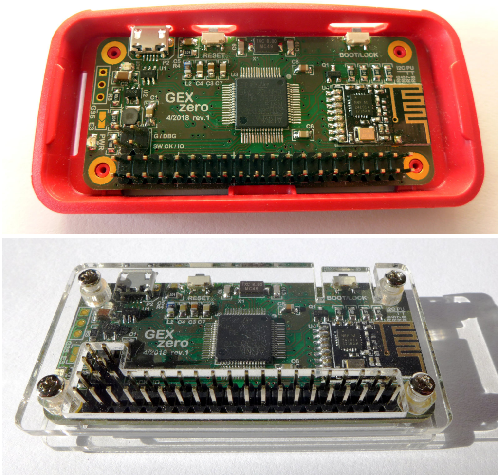
Figure 14.3: GEX Zero in the official Raspberry Pi Zero case and an aftermarket acrylic case
