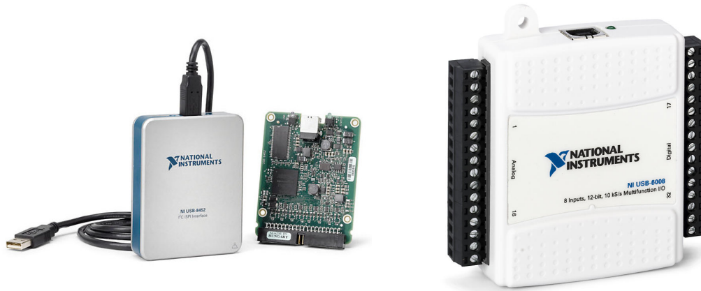
(a) : NI I 2 C/SPI Interface Device
