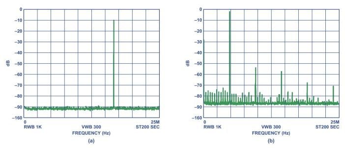
Figure 10. Output of an AD9834 with a 50-MHz master clock and (a)  $f_{OUT} = 16.667$  MHz (i.e., MCLK/3); (b)  $f_{OUT} = 4.8$  MHz.
