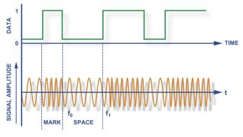
Figure 6. FSK modulation.
