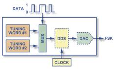
Figure 7. A DDS-based FSK encoder.
