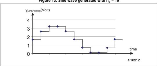
Figure 13. Sine wave generated with  $n_s = 10$
