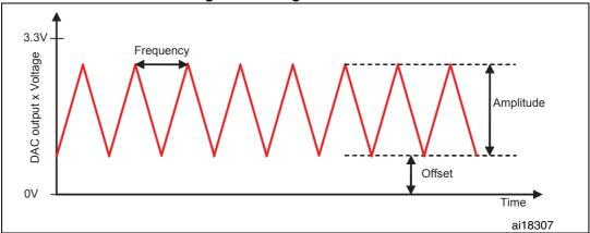
Figure 8. Triangular waveform
