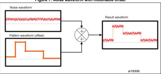
Figure 7. Noise waveform with modifiable offset
