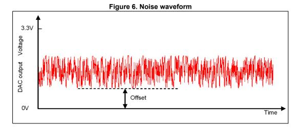
The offset (or DC bias) of the noise waveform is programmable. By varying this offset with a preconfigured table of offsets (signal pattern), the user can obtain a waveform that corresponds to the sum of the signal pattern and the noise waveform.
