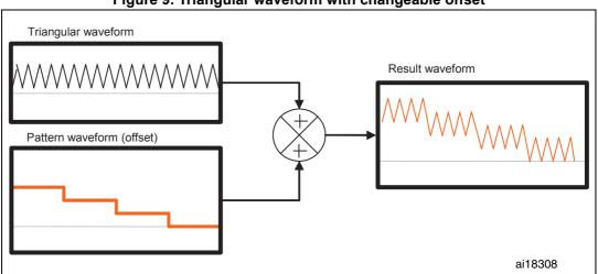
Figure 9. Triangular waveform with changeable offset
