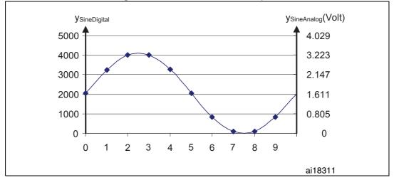
Figure 12. Sine wave model samples
