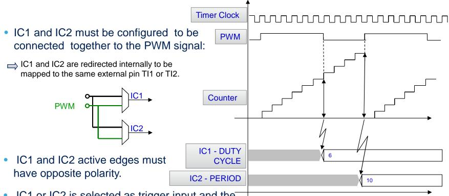
IC1 or IC2 is selected as trigger input and the slave mode controller is configured in reset mode.
