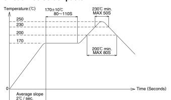
The temperature profile is based on the shown conditions. In individual applications the temperature may vary, depending on solder paste type, volume/thickness and board size/thickness. Consult your solder paste and equipment manufacturer for specific recommendations.
